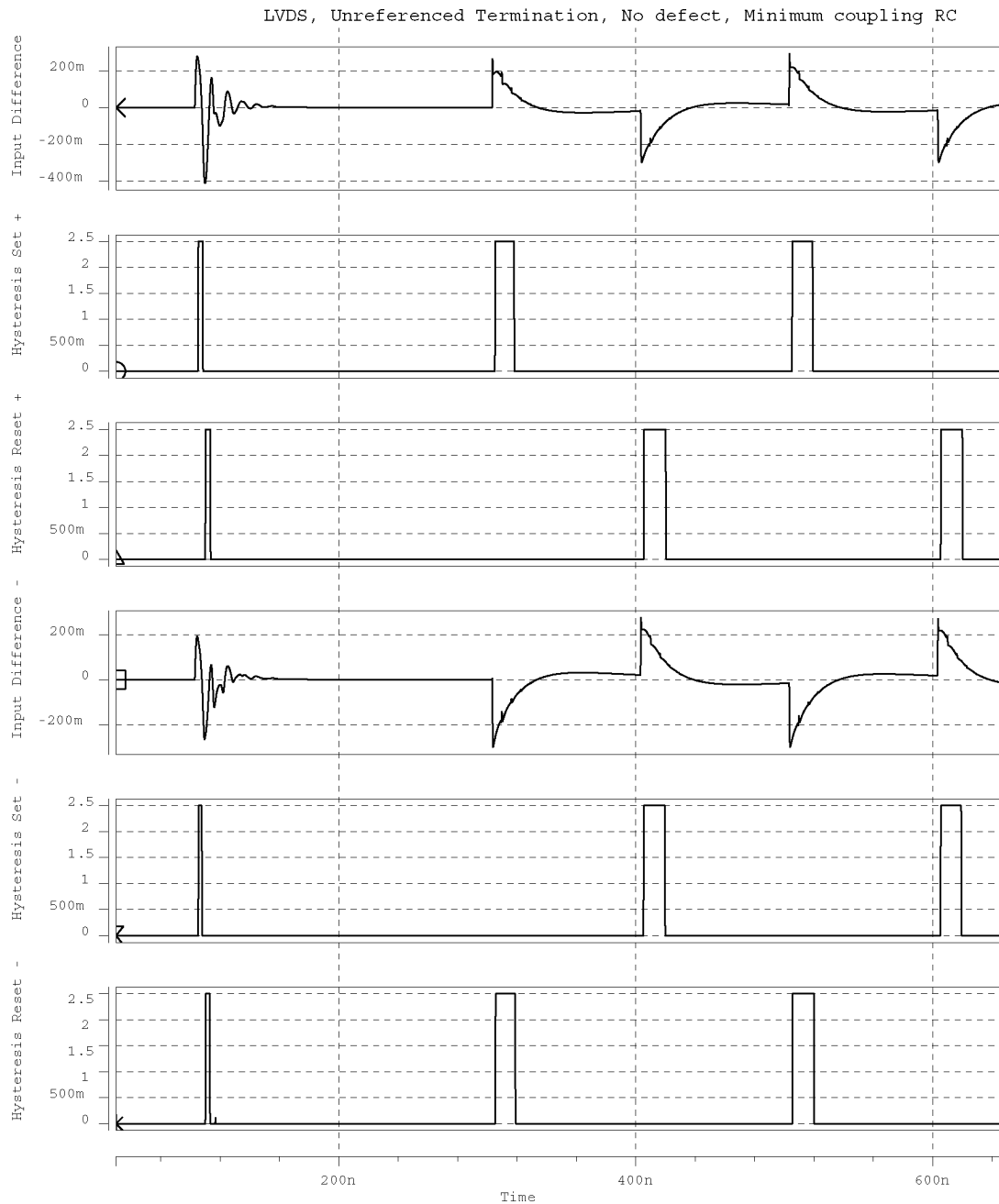
Figure D.3—Simulation of test receiver internal signals (for both legs) for the example in D.1
