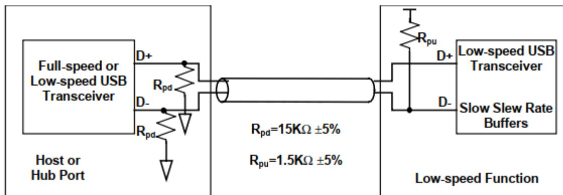
Figure 7-21. Low-speed Device Cable and Resistor Connections
