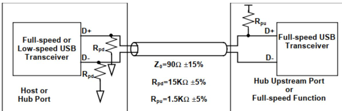
Figure 7-20. Full-speed Device Cable and Resistor Connections
